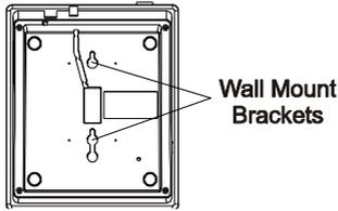
Place 2 screws into the wall then slots on the bottom of the base over the two screws heads and pull down to lock into place.
